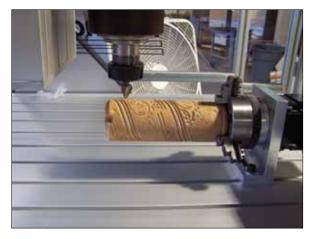
in-between each pocketing operation to rotate the part at regular intervals, typically 90°.
