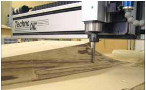
CNC automation enables you to design a part on your PC, and then reproduce that design quickly and easily using the router. There are three basic steps to this process. First, a computer image is generated, typically through a CAD program. Second, a CAM program translates the geometry of the CAD drawing and cutter compensations to output a toolpath. And lastly, the toolpath is converted to a manufacturing programming language (i.e., G-Code) used
