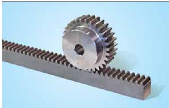
Some CNC Routers use other drive systems, such as the rack-and-pinion gear drive. The racks are typically installed on the outside of the machine, thus exposed to the elements. As the machine cuts, debris collects on the rack. These foreign materials get ground into the racks and gears, causing more friction in the drive system which, in turn, causes wear and makes the machine less accurate and unstable.
