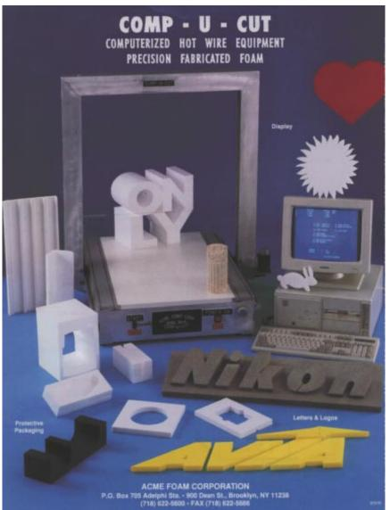
onto the table of the cutter, and press a button to download the pattern to the controller. Through the use of a PCMAC100 controller card and MasterCAM software (Techno, New Hyde Park, NY), the Hot Wire Cutter automatically cuts the pattern out of the styrofoam exactly as it was designed on the screen.
