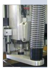
The pressure foot is ideal for plastics, woods, composites, fiberglass, or any substrate when routed. The pressure foot fits any manual high-frequency collet type spindles. This accessory can be added at any time.
