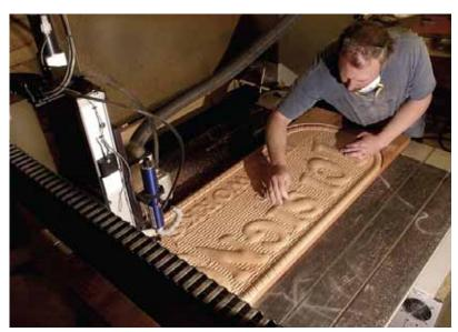
The Techno router makes it possible to produce 2D and 3D images faster and with more accuracy.
