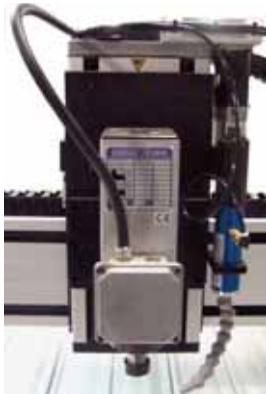
come with tool-length sensors and compensation software. This allows for the tool length to not only be measured but automatically compensated for in the G-Code software, with a simple and automatic process.
