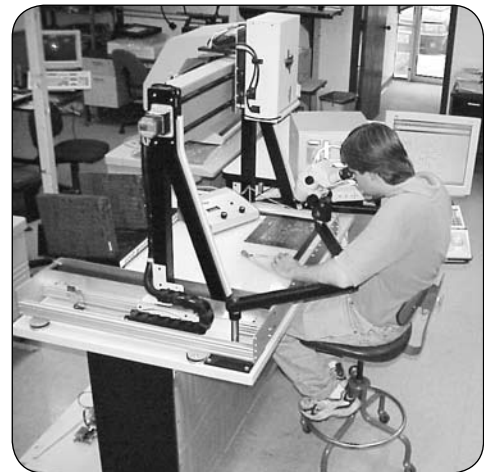
Gantry III / FB2 Table used for offline inspection of circuit boards.
