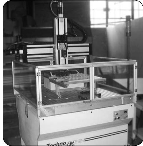
Gantry, Z-Axis for Gantry, LP Servo Controller used to place test tubes in and out of sample analyzer.
