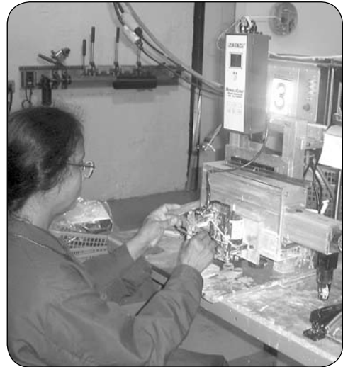
Standard-Duty Slide and Single-Axis Controller used to slice belts into stock widths.
