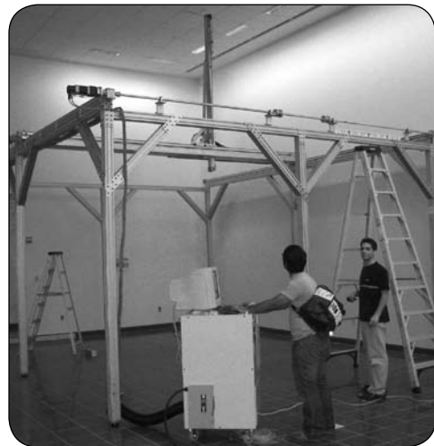
3-Axes open frame Belt Slide with HP Servo Electronics. Used to test obstacle avoidance for unmanned drones.
